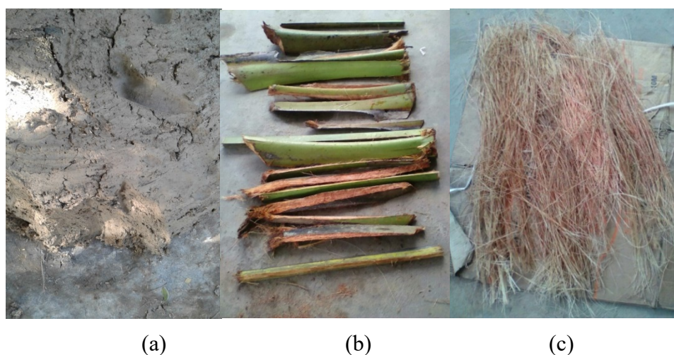
Figure 1 (a) Mixture of soil and paddy shell (b) Strips of Corypha palm's stem (c) Dried coryphe fibres
